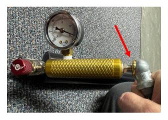
You might need a small, bladed screwdriver or a core tool to depress the Schrader valve core in the <a href="INF-KIT">INF-KIT</a> to let gas out if it is above 250 psi.
